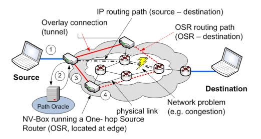
Figure 6: Routing Overlay using One-hop Source Routing
