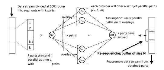
Figure 8: Transmission Mechanism
