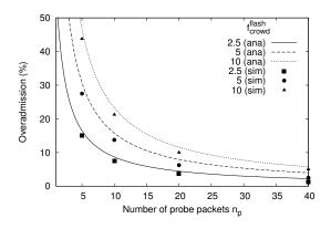
Fig. 4. Analytical overadmission depending on the number of probe packets  $n_p$  and the flash crowd factor  $f_{crowd}^{flash}$ . The lines are validated with simulation results.
