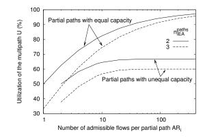
Fig. 7. Multipath routing prohibits full utilization of partial path capacities for IEA-based AC.
