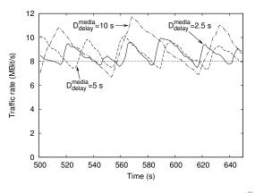
Fig. 8. Initial constant media delay and a flash crowd factor of  $f_{crowd}^{flash} = 5$  lead to oscillating admitted PCN rates and temporary overadmission.
