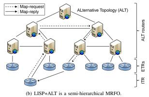
Fig. 6. LISP currently uses LISP-MS with LISP+ALT.
