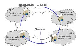
Fig. 7. LISP-DHT uses a modified Chord-ring as a MRFO.
