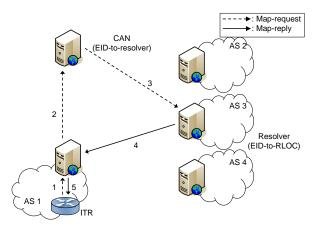
(a) DHT-MAP: map-requests are served by AS-local resolvers (bottom-level mapping systems). If the resolver cannot find the requested EID in its own database, it forwards the map-request over the CAN (top-level mapping system) to an appropriate resolver in another AS which answers the query.
