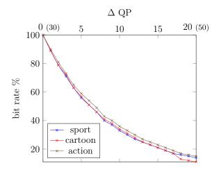
Figure 8: Adaptation through adjustment of transform coefficient quantization.
