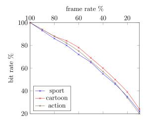
Figure 6: Adaptation through frame rate reduction.
