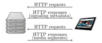
Figure 3: Principle of adaptive HTTP streaming.
