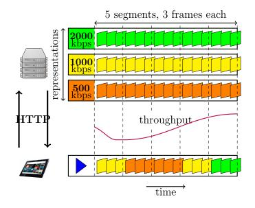
Figure 4: Video representations available for adaptive HTTP streaming.
