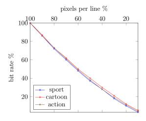
Figure 7: Adaptation through resolution reduction.
