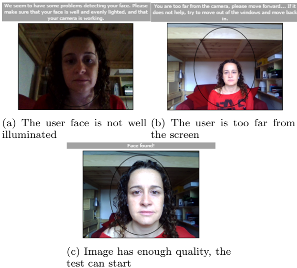
Figure 2: On-line monitoring of test conditions: distance from the face to the camera, image quality and lighting conditions are checked and feedback is provided to the user.
