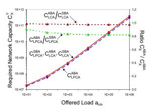
**Fig. 4.** Bandwidth savings with ABA for different traffic demand models
