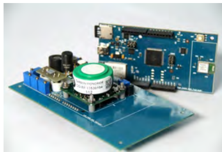
Fig. 7.1 The Arduino board of the sensor box.
