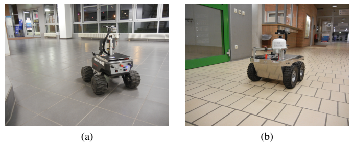
Fig. 9: Multi-SLAM with two cooperating robots. Image showing “Simon” (a) and “Georg” (b) during the multi-SLAM experiment.
