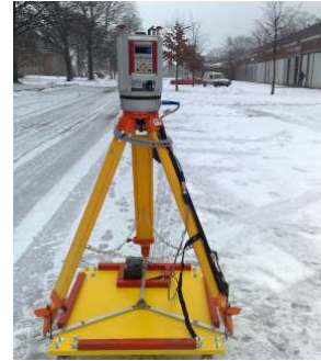
Fig. 1: The Riegl VZ-400 3D laser scanner mounted on a tripod and a self assembled dolly. The scanner has manually moved to different positions as the campus of Jacobs University Bremen.
