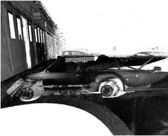
Fig. 7: Correct registration using SIFT features. The change in the scene does not have an effect on the registration quality.
