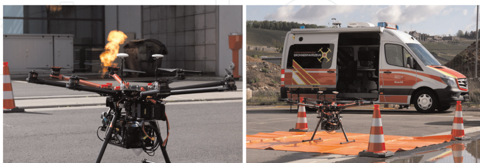
Figure 2. UAV with mounted mapping payload in front of simulated facade fire (left) and the firefighter command vehicle (right).
