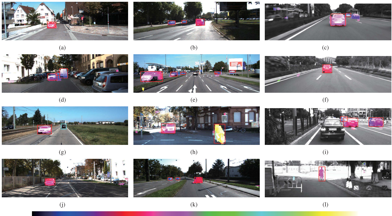
Fig. 8. The results of KITTI datasets are displayed in column 1 and 2. The results on SYSU datasets are displayed in column 3. The bottom color bar stands for the disparity from large to small.
