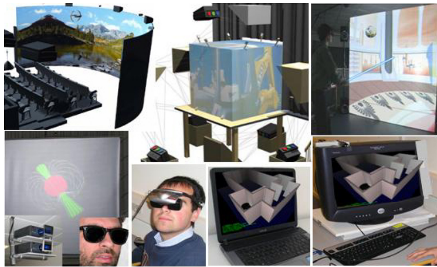
Fig. 1. Virtual Reality facilities at Aalborg University VR Media Lab and Medialogy Copenhagen. Top from left: 160deg Panorama; 6-sided CAVE; 1-sided CAVE. Bottom from left: Small Powerwall with projectors and filters; HMD; 3D Laptop, 3D Desktop.
