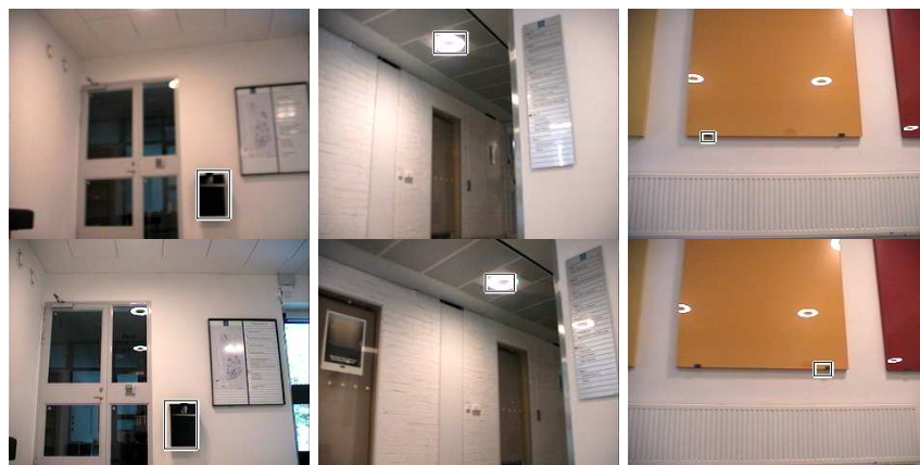
Fig. 2. Matching results in loop closing situations: the first row shows a ROI in a current frame, the second row shows a previously seen ROI from the database. This situations usually occurred after the robot drove a circle and revisited the same area again. Two correct matches (left, middle) and one false match (right) are shown.
