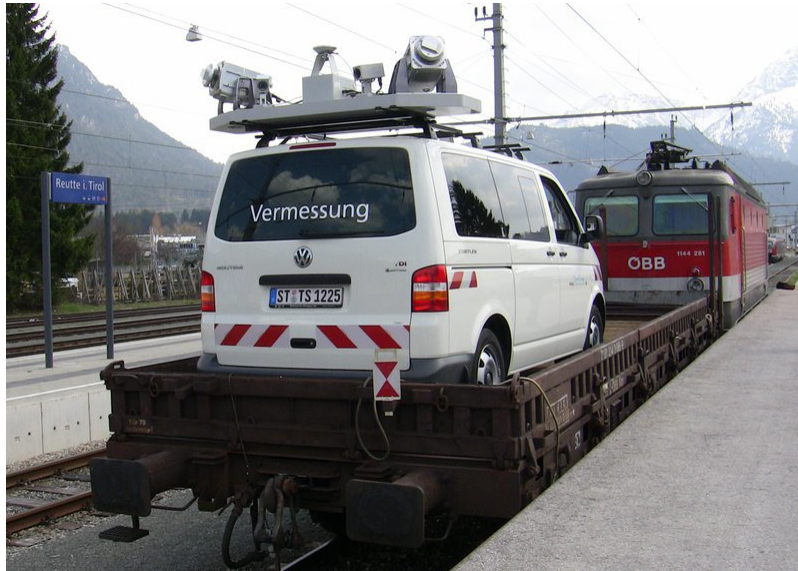
Figure 11: The Optech Lynx Mobile Mapper on the back of a train wagon.
