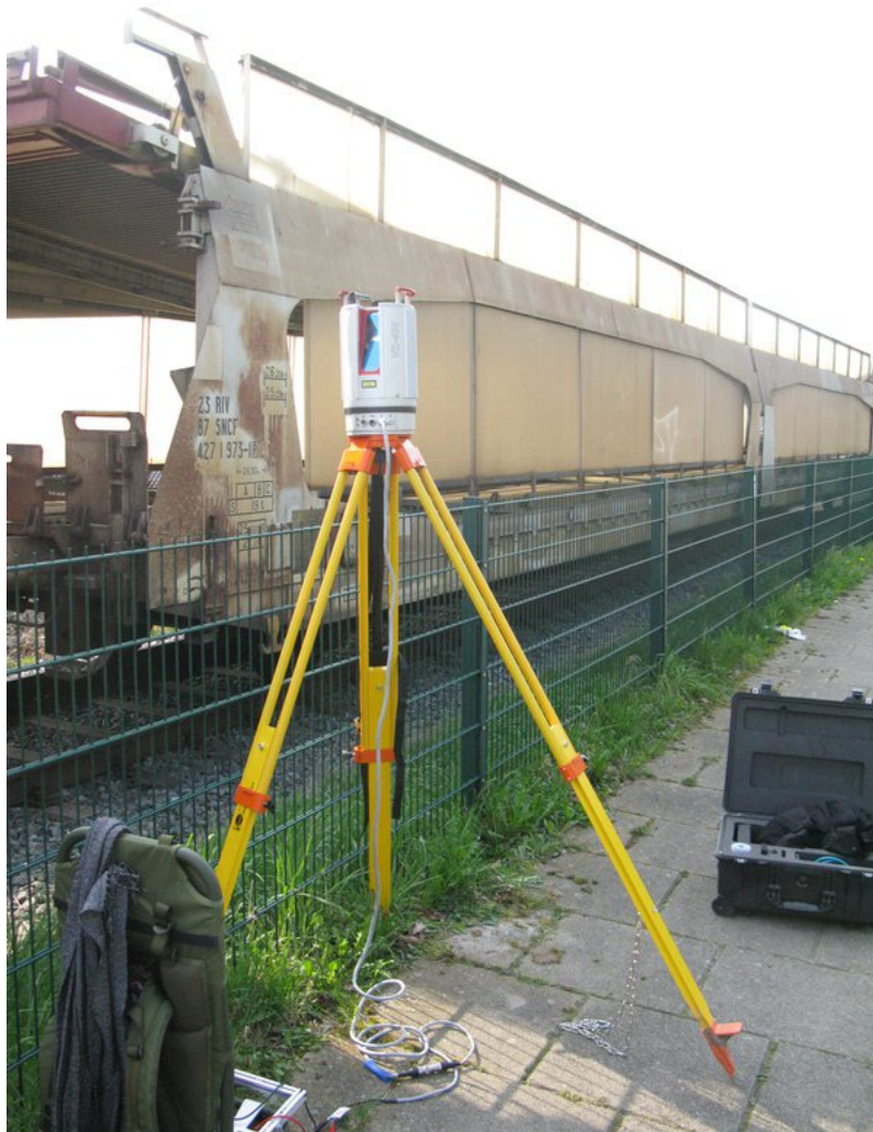
Figure 13: The Riegl VZ-400 laser scanner set up next to the train wagon.
