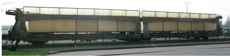
Figure 12: A photo of the scanned train wagon with a bogie distance of 20 m.
