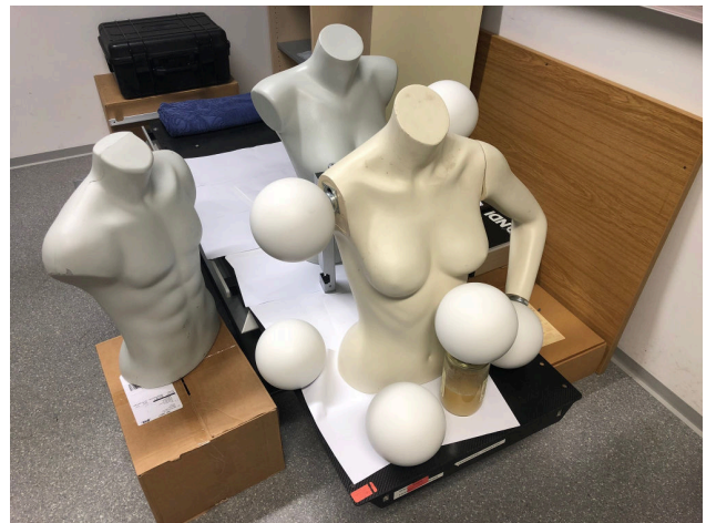
Figure 4. Sample scene with six calibration spheres. Phantoms are added for texture and variation.
