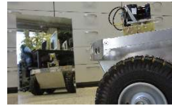
Fig. 1: Robot equipped with the 3D-Hokuyo multi-echo laser scanner facing an unframed mirror.
