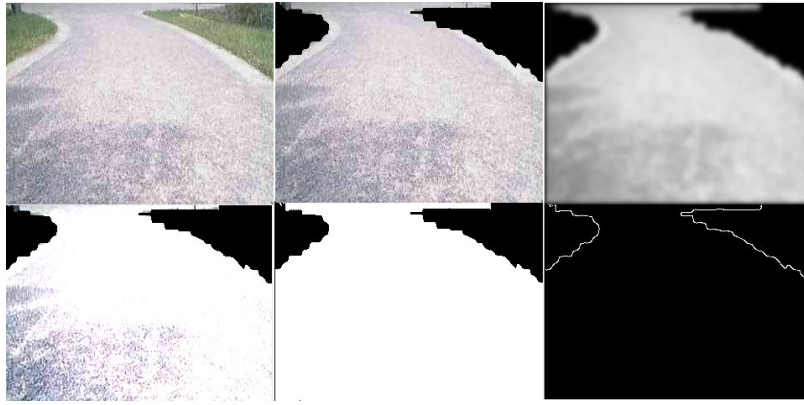
Figure 3. Processing steps for border extraction: The figure shows an original webcam image and the steps after applying the following filters: green to black, gaussian blur, contrast enhancement, thresholding and border extraction.
