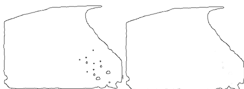
Figure 4. Detected borders after edge detection (left) and object extraction(right).
