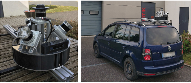
Fig. 2. Left: LiDAR scanning rig with four Ouster laser scanners. Right: Rig mounted on the car of the corresponding author.
