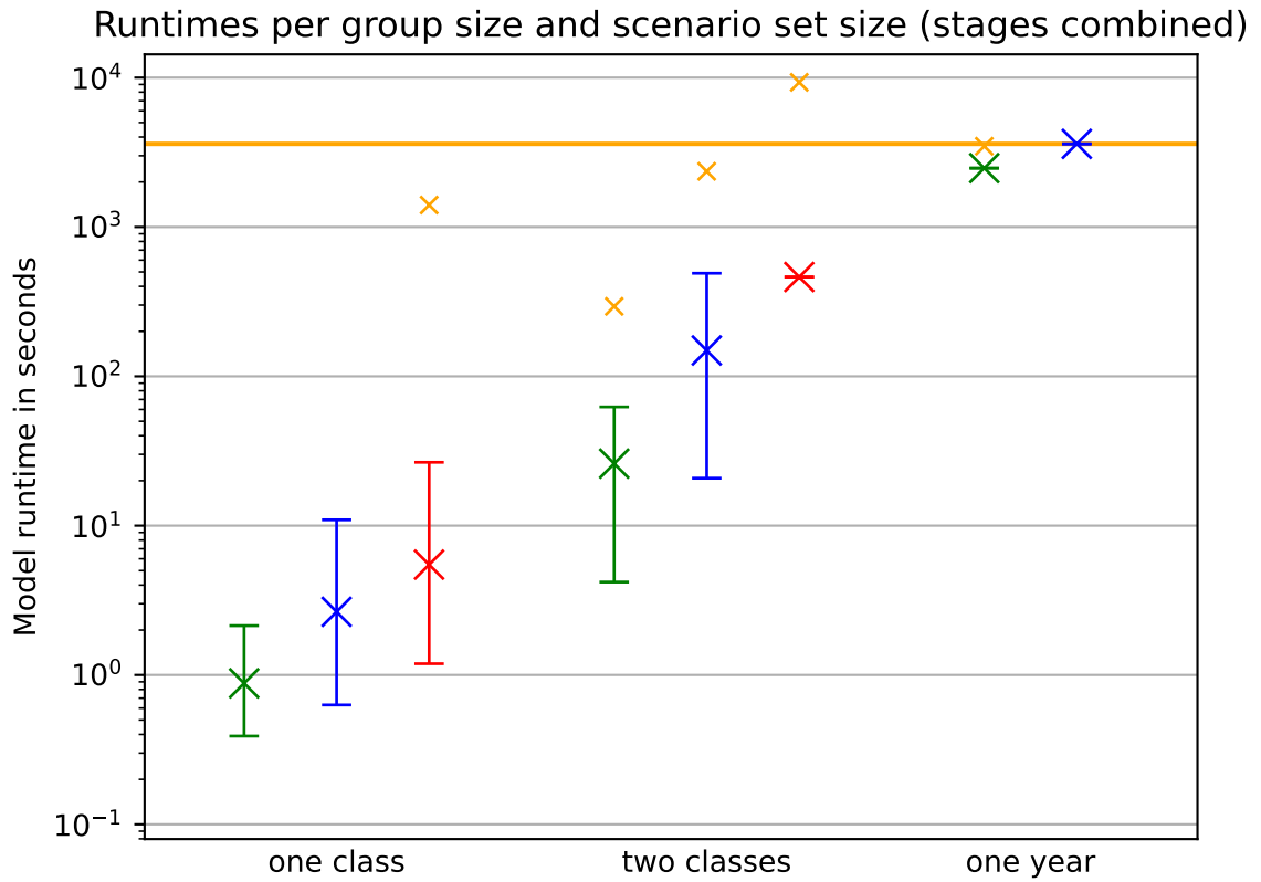
Fig. 8.2: The figure shows the runtimes of second iteration instances with the objective function optimizing for both stages combined, showing the average, maximum and minimum outcomes. Green elements are instances with five scenarios, blue elements represent instances with 15 scenarios and red elements stand for 30 scenario instances. The horizontal line in orange is at the imposed time limit of 3600s. Note that experiment with only one available data point have very high loading times and in theory hit the time limit before the model was ready to begin calculation. For more precise numerical values as well as the number of instances run for each data point refer to Table 9.1 and Table 9.4
