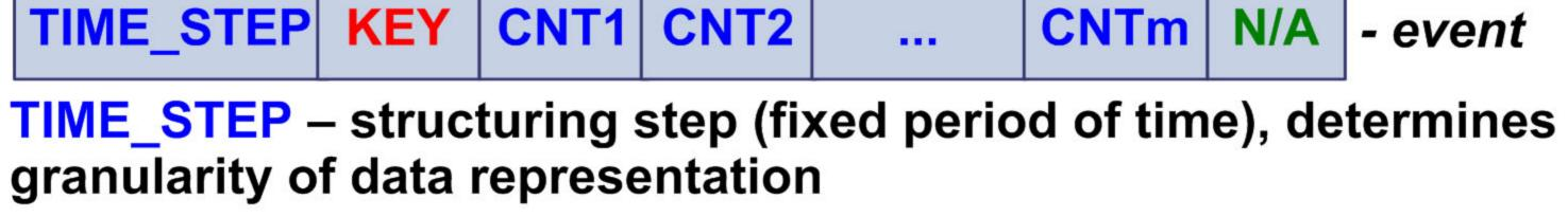
CNTi – simple / conditional counter on packet header field, grouped by KEY (for example, packets number, traffic volume, etc.)
