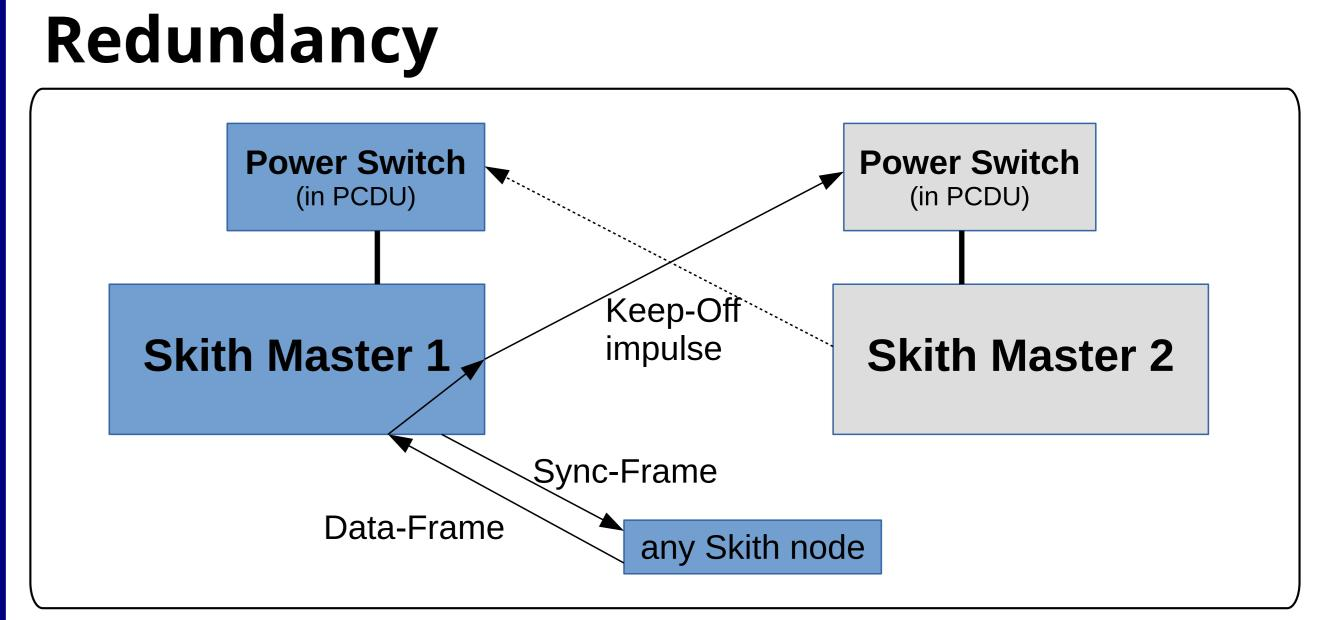
Redundancy mechanism of SKITH Master Nodes
