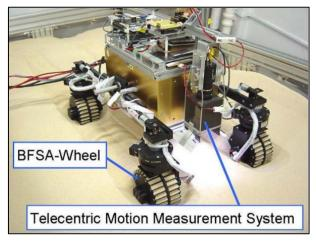
Source: Nagatani et al., Accurate estimation of drawbar pull of wheeled mobile robots traversing sandy terrain using built-in force sensor array wheel
