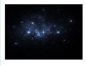
In our Space Manoeuvre Simulation Facility we use air bearing vehicles on a glass plate. Below this glass plate we have a starry sky with 3000 Stars. We shall use a camera to look a small segment of thy simulated sky, and using similar methods like star sensors we determine our position (2D) and attitude (1D).
