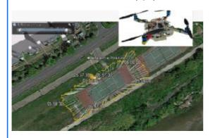
Precise localization of quadrocopters will be implemented and evaluated using GPS. Provided GPS-position and GPS-raw-data will be transmitted to a base station. For cooperative flights we use two or more quadrocopters and compute their relative pose using differential GPS.
