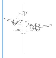
Down on earth it is barely possible to test the 3D rotation of satellites. Therefore we build air bearing spheres that contain all the necessary components like sensors and actuators in order to design and test a real life 3D attitude control.
