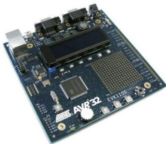
Abb.: 27 ATMEL EVK1100 (ELMICRO Computer GmbH)
