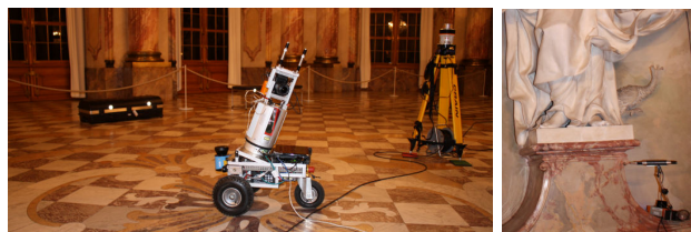
Fig. 1. Irma3D in the Imperial Hall of the Würzburg Residence. Visible in the background is one of the transmitters of the iSpace localization system and a box with two of the reflective targets used for calibration. The handvector bar is used to measure distinctive points in the environment that are used to evaluate the quality of the final model.
