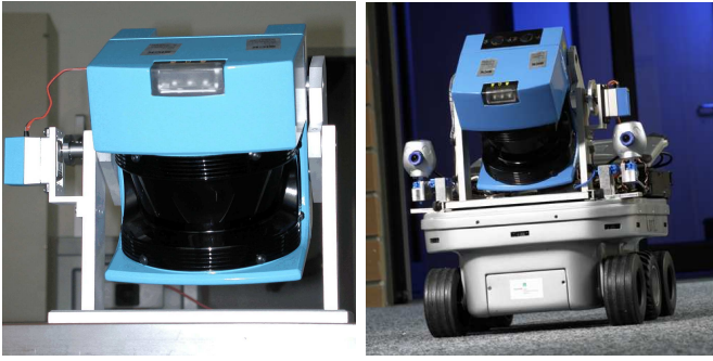
Fig. 1. Left: The 3D laser range finder. Its technical basis is a SICK 2D laser range finder (LMS-200). Right: The autonomous mobile robot Kurt3D.
