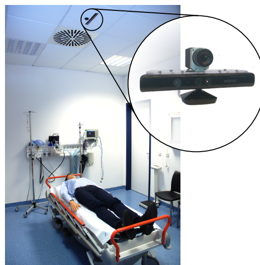
Fig. 1. Emergency room at the Universitätsklinikum Erlangen with Microsoft Kinect and Optris PI400 (not used in this paper) mounted on the ceiling.
