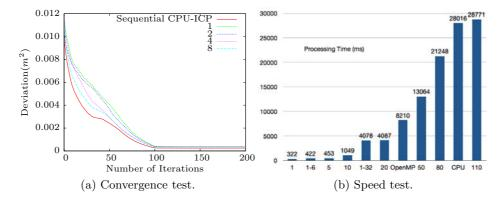
Fig. 4: The result of the 3D registration experiment of 68229 points. 1-6 means the queue length is increased gradually in iterations as follows: 1, 2, 3, 4, 5, 6, and 1-32 as: 1, 2, 4, 8, 16, 32. It is observed from the speed test that GPU-ICP is 88 times faster than the sequential CPU-based ICP.
