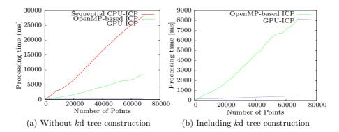
Fig. 6: The runtime comparison among sequential CPU implementation, OPENMP-based implementation and GPU-ICP.
