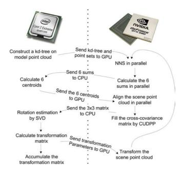
Fig. 2: The coordination between CPU and GPU in the GPU-ICP algorithm. Notice that other than constructing the k-d tree, CPU does only negligible work. The data transfer over the PCIe is minimized. Pictures of the chips are taken from manufacturer websites.
