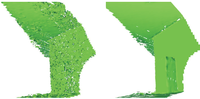
Fig. 4. Influence of the normal estimation quality. Consistent normals result in connected surfaces (right) while inaccurate estimations produce holes in the triangle mesh (left).
