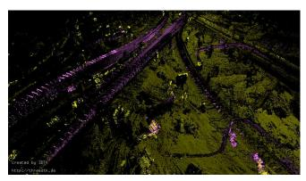
Fig. 1: crossroad from KITTI scene 51 with moving objects in magenta and static objects in yellow
