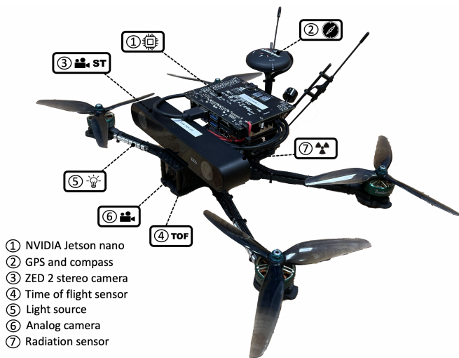
Fig. 4. Overview of the UAV hardware concept.
