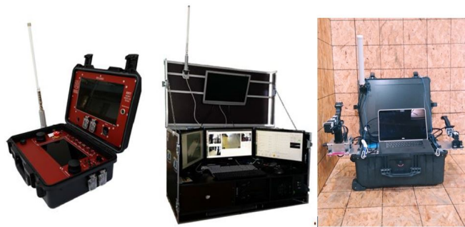
Fig. 5. Different types of operator stations for visualization of 3D map, live camera views and radiation value display.
