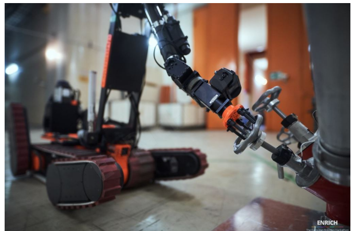
Fig. 8. Previous version of Hurrigan with 6-DOF arm and simple valve tool.
