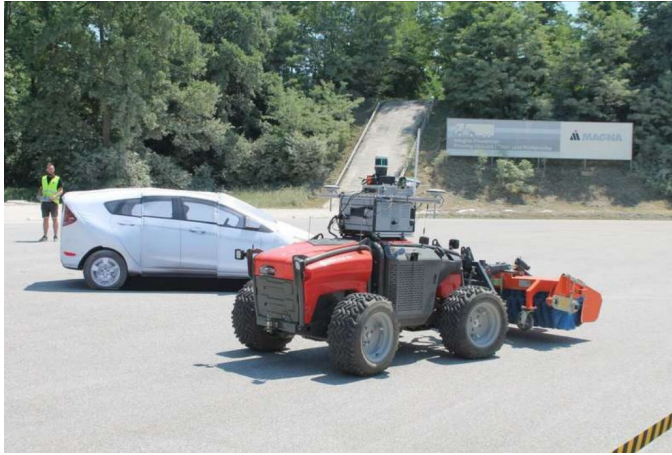
Fig. 3. Collision scenario when using the automated equipment carrier with sweeper at the Digitrans test track
