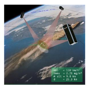
Fig. 1. The 3 cooperating TOM satellites [8] for threedimensional characterization of ash clouds from volcano eruptions.
