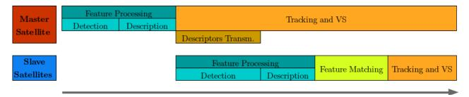
Fig. 5. Image processing pipeline for target tracking and image based visual servoing.
