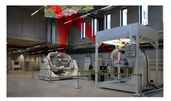
Fig. 8. Cameras mounted on the two precision turntables to simulate the orbit motion in imaging the 3D-object on the ceiling.
