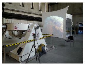
Fig. 8. Simulating Image Based Visual Servoing of a single satellite with a precision turntable.
