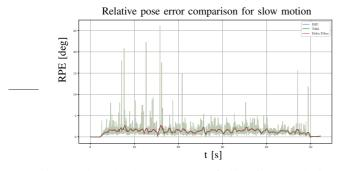
Fig. 9: The relative pose error of all estimators during slow motion over time. The Savgol-filter is applied with a window size of 51 and a polynomial degree of 3 to remove the effect of outliers. In the background the noisy pre-filtered errors are shown with low opacity.
