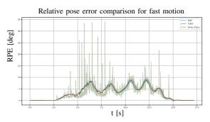
Fig. 7: The relative pose error of all estimators during fast motion over time. The Savgol-filter is applied with a window size of 51 and a polynomial degree of 3 to remove the effect of outliers. In the background the noisy pre-filtered data is shown with low opacity.
