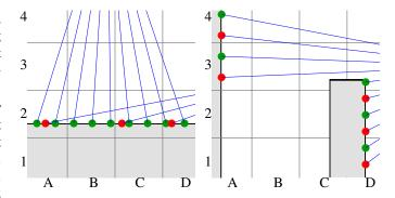
Fig. 3. Two examples for false positive when applying a naive approach to find dynamic voxels. See Figure 2 for a legend. Left: Due to the surface being scanned at a shallow angle, the scan measuring the red points will wrongly mark voxel B2 as free when traversing the line of sight up to the red point in A2. Right: Due to the tip of the structure in D3 only measured by the green scan, it will be wrongly marked as free when traversing the line of sight up to the red point in A3.
