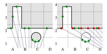
Fig. 2. The gray raster marks the 2D voxel boundaries. Blue lines mark the scanner lines of sight. Gray areas mark solid space while white areas mark free space. Round green and red dots represent the measured scan points of the first scan (left) in green and of the second scan (right) in red. The circular object in areas C1 and C2 is dynamic and only measured by the first scan (green points in C1 on the left). Dotted lines represent the former location of the circular object.
