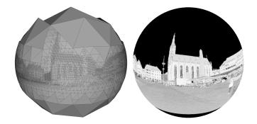
Fig. 5. Left: Visualization the nodes of a sphere octree from a terrestrial scan. Right: reflectance values of that scan as a texture on a sphere in the same orientation.
