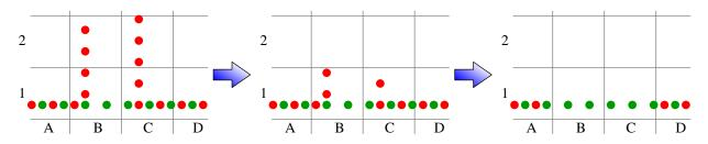
Fig. 6. Left: original two scans. Center: Voxels B2 and C2 found to be see through and cleared, artifacts remain in B1 and C1. Right: Red points from voxels adjacent to freed voxels B2 and C2 also get removed, leaving a smooth surface
