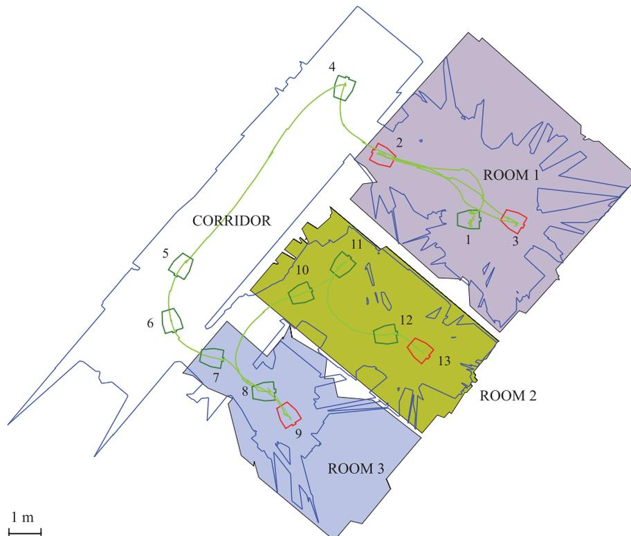
Fig. 6. Robot path and scanning positions during exploration.
