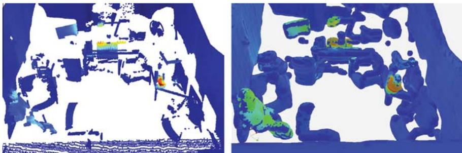
**Fig. 12.** Image of a point cloud (left) captured at scan position 12 in office room 3 and the reconstruction (right).
