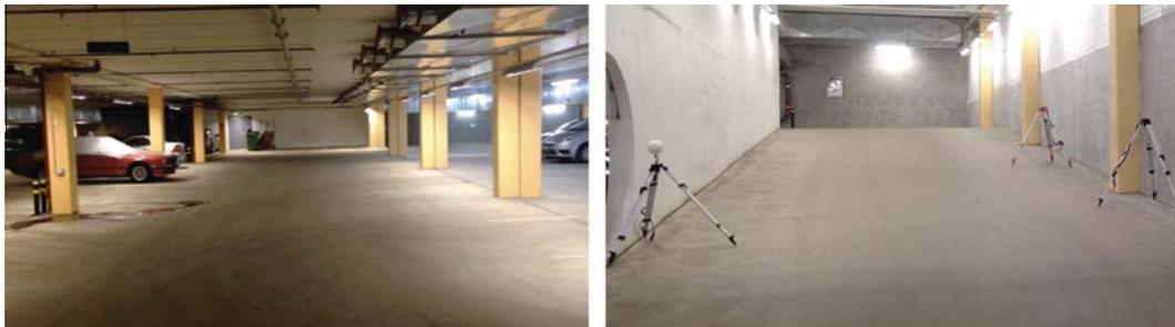
**Fig. 5.** Images of the indoor environment. Left: On each floor, the visibility is dozens of meters in multiple directions. Right: The ramp is sloped vertically by 5.7 deg, and has a more limited visibility. Tripods for the reference TLS scans are shown.
