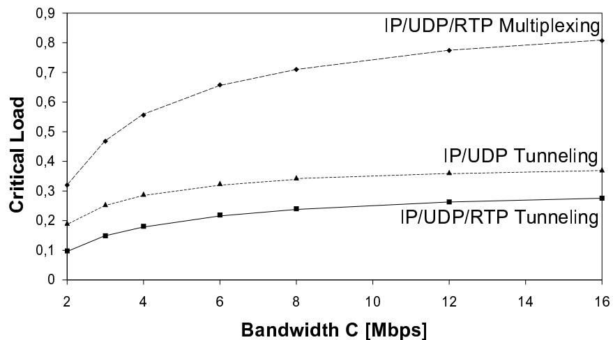
Figure 5: Impact of the bandwidth on the critical load
