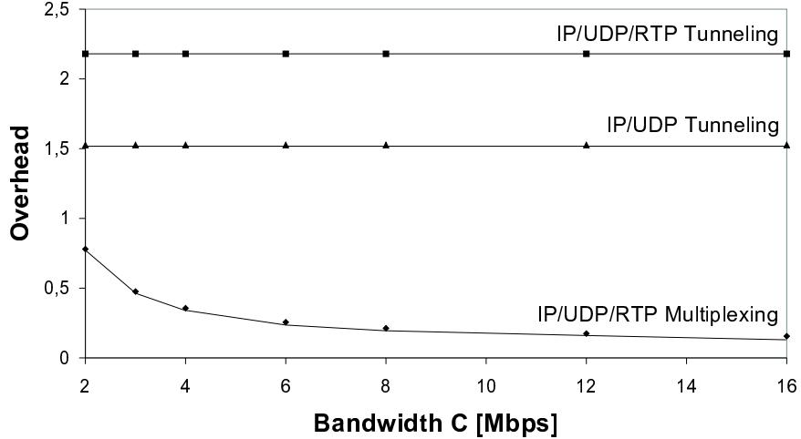
Figure 6: Impact of the bandwidth on the protocol overhead
