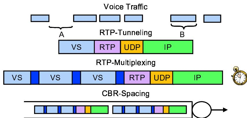
Figure 2: Multiplexing and tunneling of voice samples with spacing
