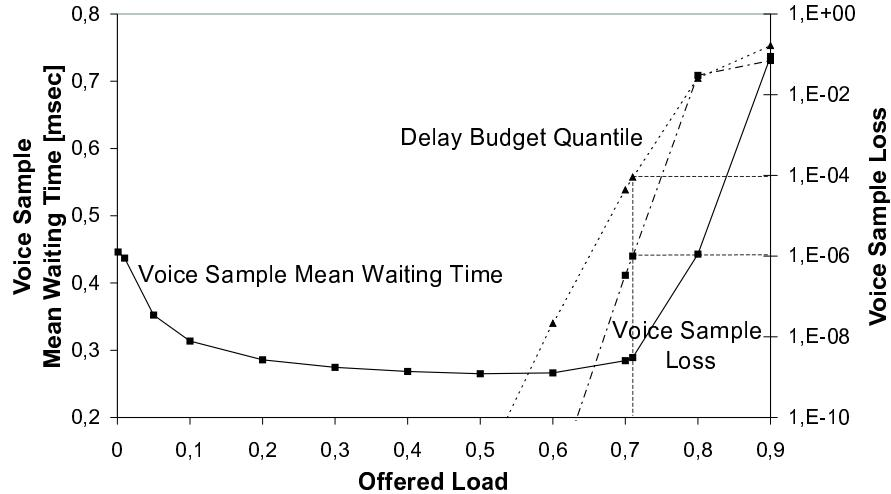
Figure 4: Impact of the offered load on the voice sample mean waiting time, the delay budget quantile, and the loss probability
