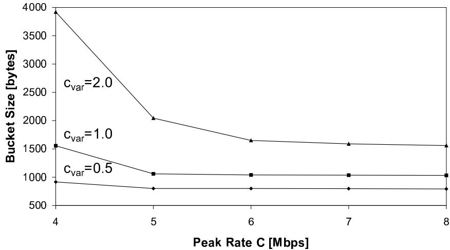
Figure 7: Impact of the peak rate on the leaky bucket size
