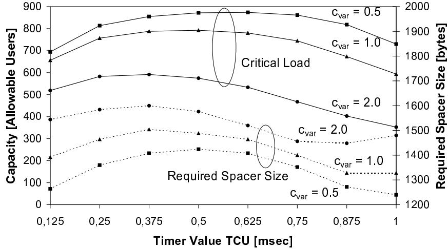
Figure 3: Impact of timer setting on the capacity and the required spacer size
